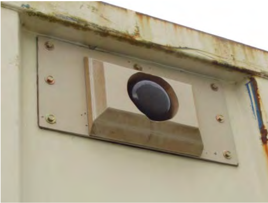
Figure 2.6 An image of the container used in the field trials. One of the two GPS units can be seen on the side wall, just below the ridge, near the open door. The other GPS unit was positioned on the other side wall at the back of the container.
