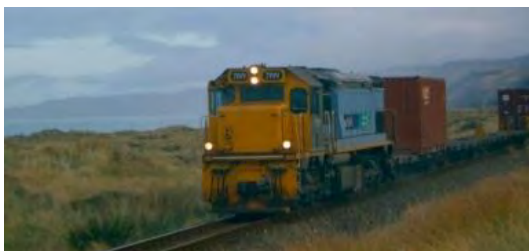
Figure 6.2 Mainline container train hauled by DX locomotive
