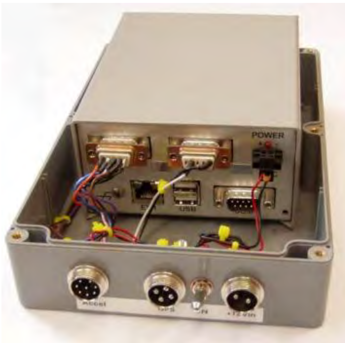
Figure 2.2 An image of the ARM log (also referred to as the Armlog) data acquisition unit
