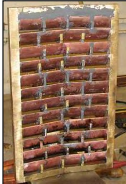
Figure 3.6 Type 16 Grate During Fabrication
