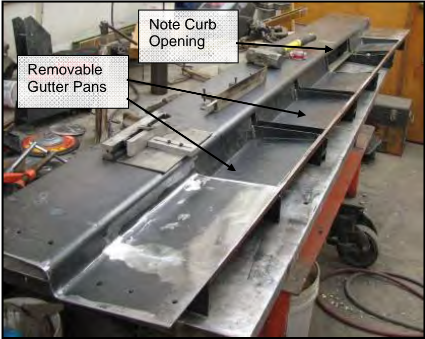
Figure 3.4 Combination Inlet Gutter Panel During Fabrication (Type 13 and 16 grates)
