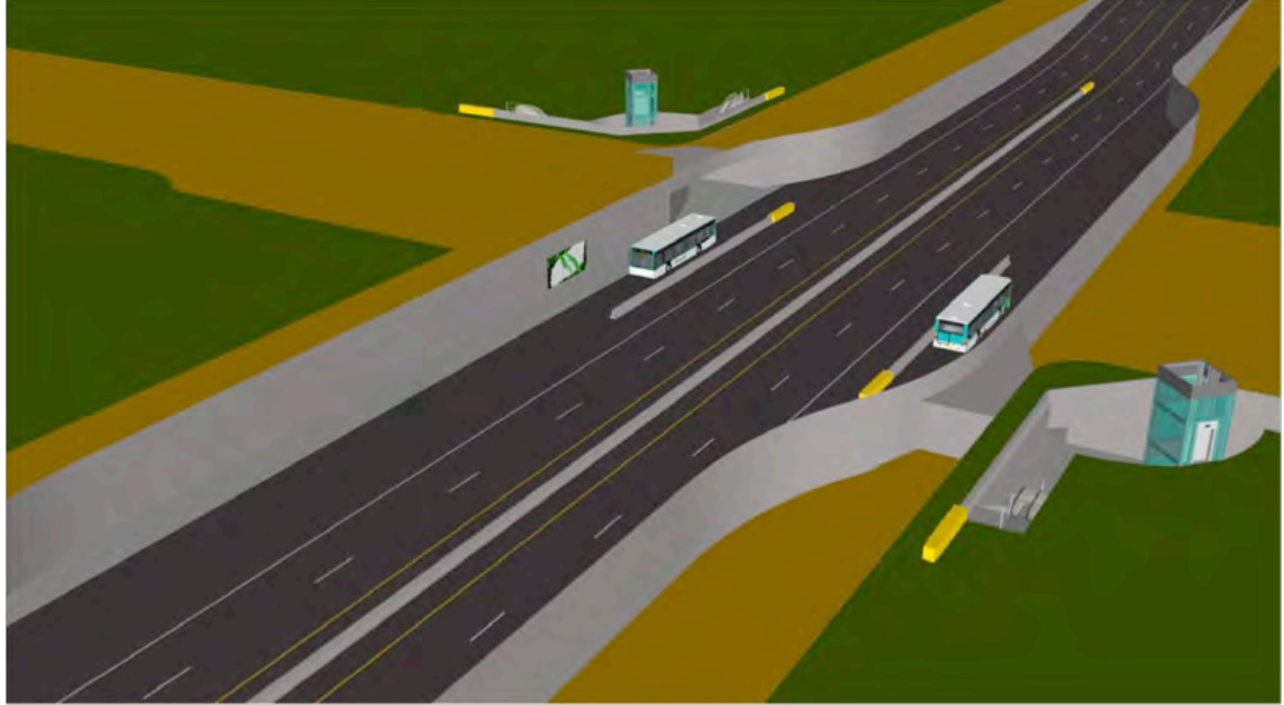
Figure 9: Underpass Bus Transfer Station Concept (Cutaway View)
