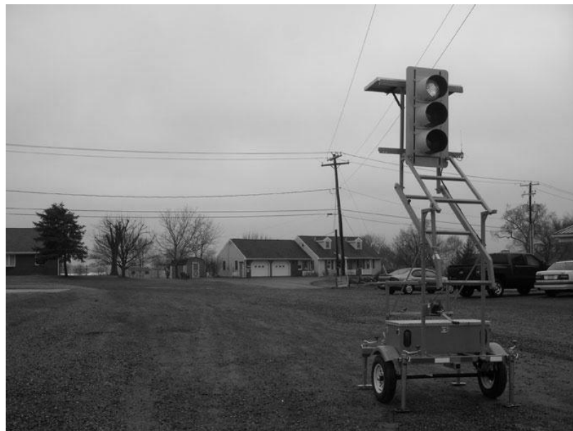
Figure C.2. Temporary signal lighting
