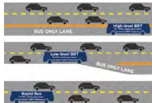
Page 16: Rapid Bus, Low-Level BRT and High-Level BRT graphic by Irving Pham, Reconnecting America
