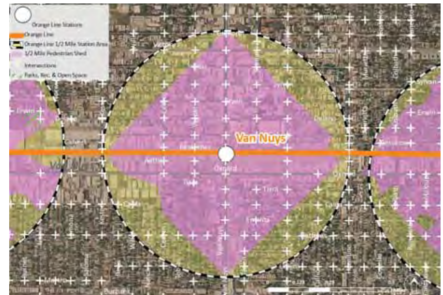
1/2 mile Walkshed (Source: LA County, Design Community and Environment, and Reconnecting America)
