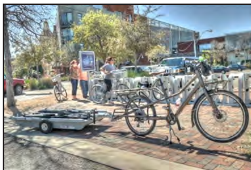
Figure 28. San Antonio B-cycle Rebalancing Vehicle Towed by Electric Bicycle
