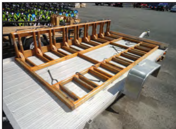
Figure 27. Custom-Made Rebalancing Trailer, Nice Ride Minnesota
