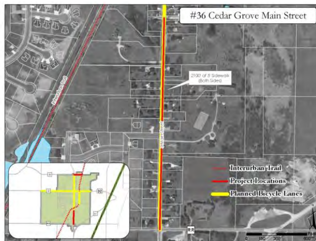
Figure 36: The Project Adds Sidewalks, Bicycle lanes, and Sharrows in the Village of Cedar Grove (source: Sheboygan County NOMO)
