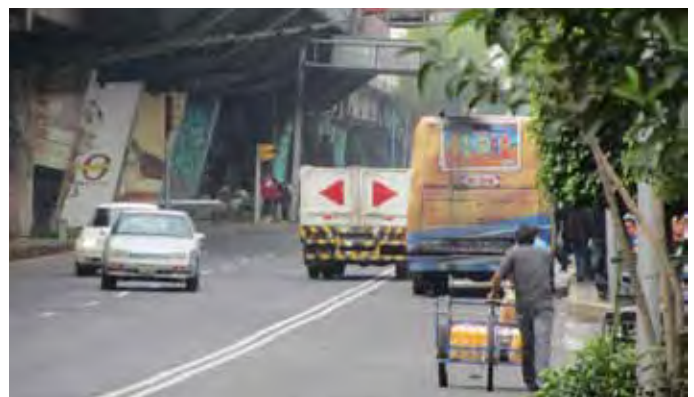
A curbside counterflow lane on Eje 2 Oriente in Mexico City (the street has a southbound bus lane and five northbound lanes, though only two can be seen in this image). The small truck had been driving southbound illegally on the bus lane, and then attempted to overtake the bus as it stopped at the station. Northbound cars are trying to get out of the way. Also note the pedestrian carrying merchandise in the bus lane. Photo by Carsten Wass.
