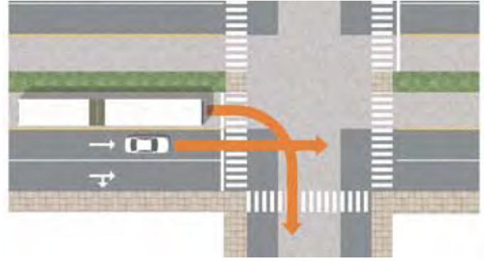
Crash diagram illustrating a potential conflict between right turning buses and vehicles continuing straight. This type of crash has been reported on TransMilenio.
