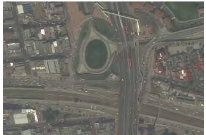
Junction between three TransMilenio corridors: NQS, Calle 80, and Avenida Suba. Bus connections between the three corridors are done via overpasses and underpasses, which maximizes capacity for all the movements and minimized potential conflicts between buses. Google Earth image.
