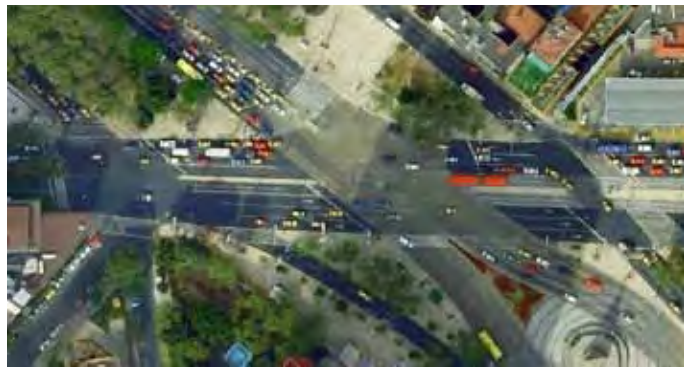
A wide, complex intersection along Metrobus Line 1 in Mexico City. This type of design has more safety issues than the simple, narrow intersection in the image above. Google Earth image.
