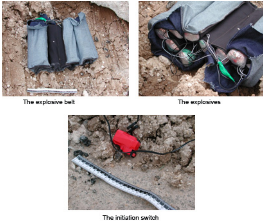
Figure 12: Components of the IED
