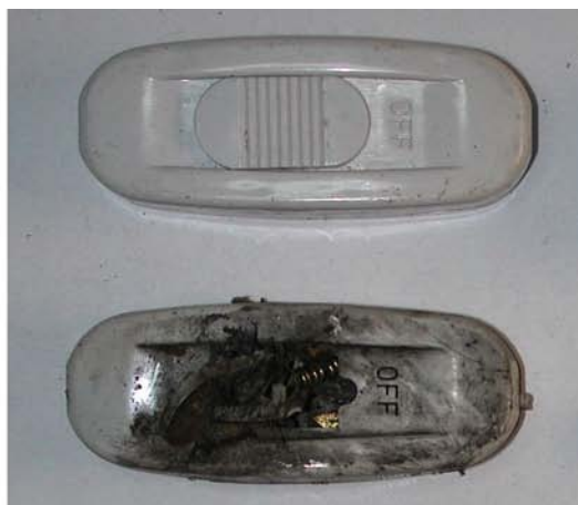
Remains of electrical initiation switch (shown below a similar switch)
