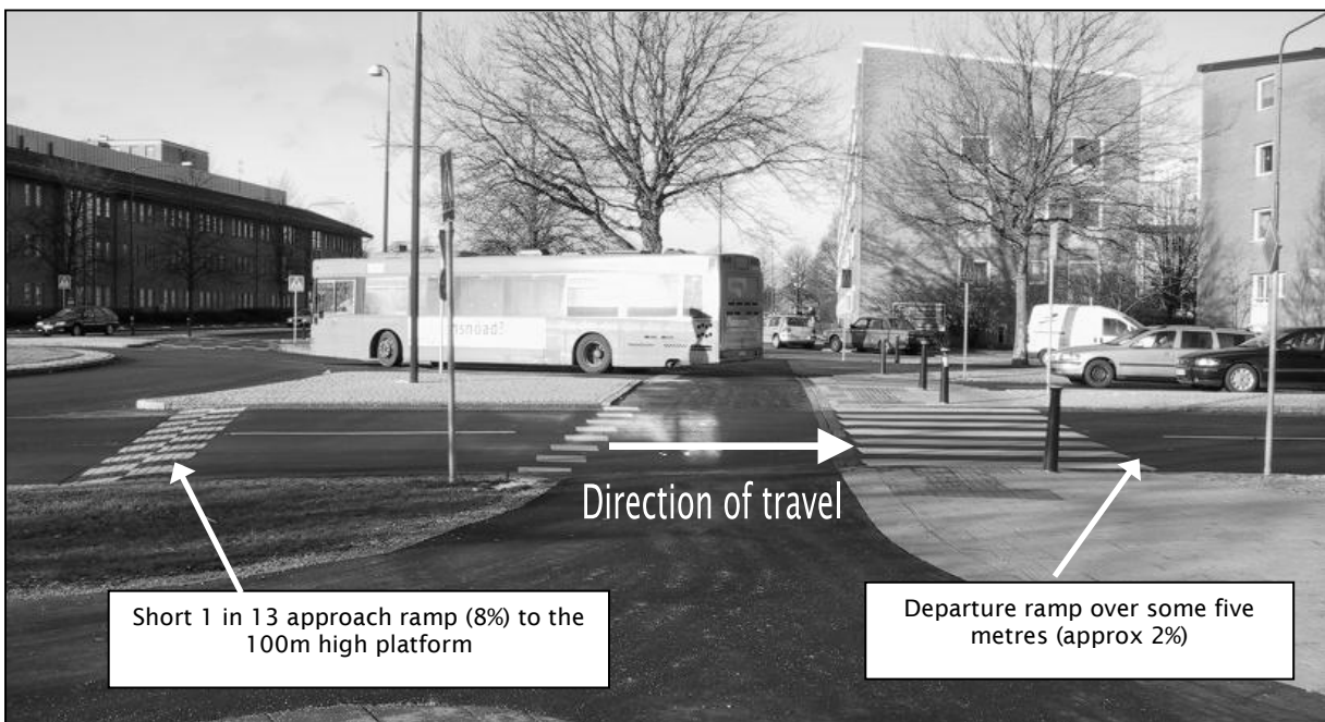
Figure 7.31 Side view of a platform from the Swedish city of Malmö with roundabout exit lanes in the foreground. For entry lanes in the background, this profile is in the opposite direction of vehicle travel. A median island of some length is required to allow for the differing carriageway levels in each direction (photo provided by Transport Department, City of Malmö)
