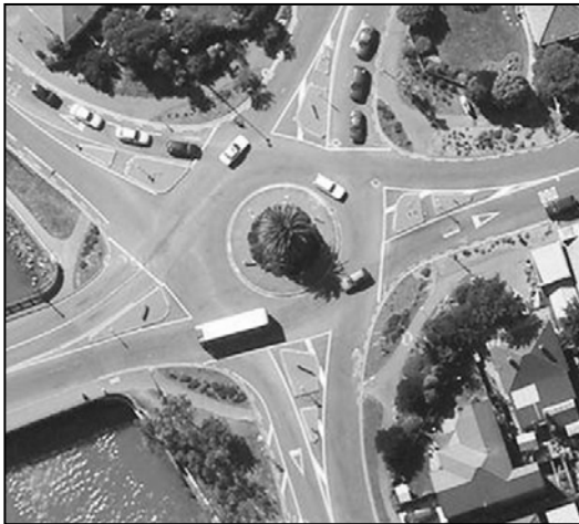
Figure 3.10 Example of a roundabout built with minimal regard for speed control: Pages Road, New Brighton Road, Owles Terrace and Seaview Road in Christchurch (photos courtesy of Google Maps)
