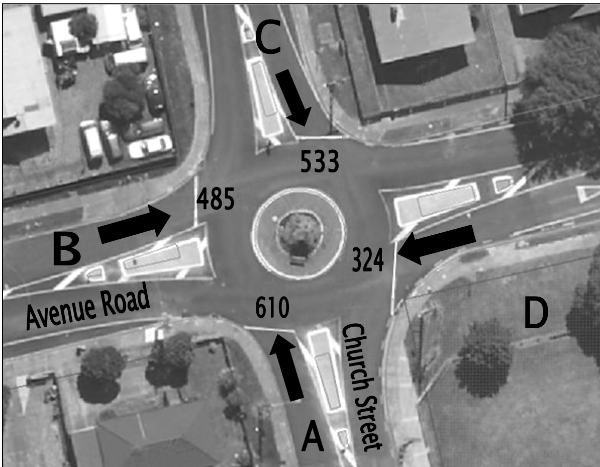
Figure 4.15 Diagram showing counted total traffic volumes between 9:30am and 3:00pm on one sample weekday
