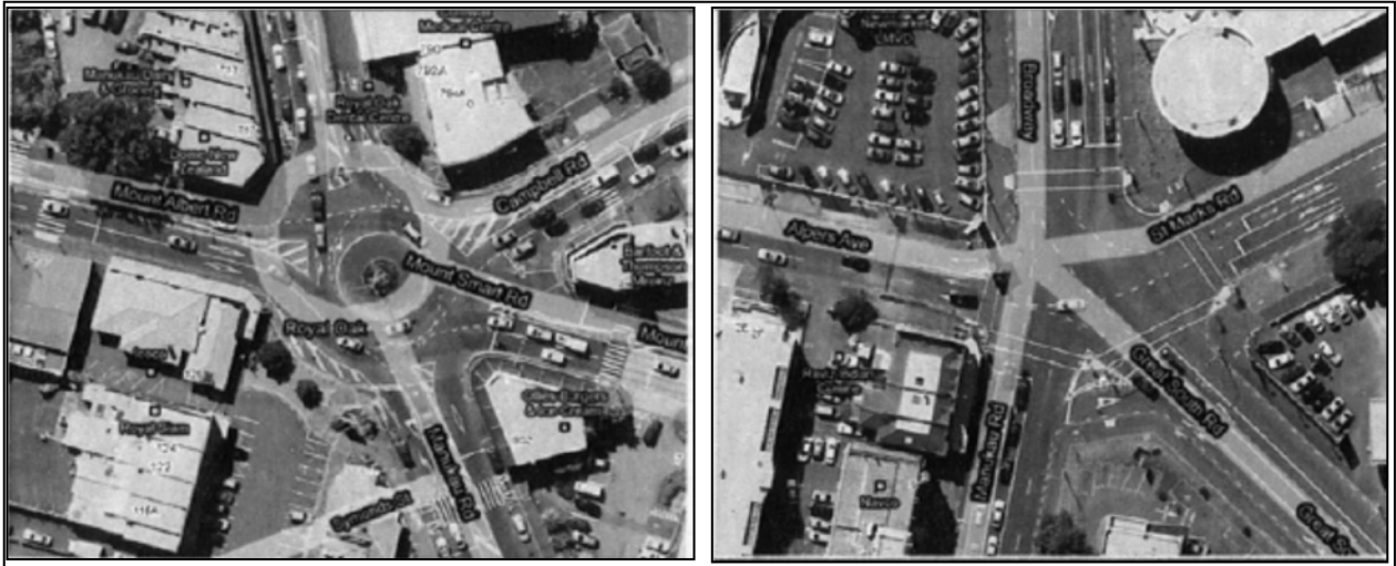
Figure A3 Matched pair 1: Manukau Road–Mt Albert Road roundabout (left) and Manukau Road–Broadway traffic signals (photos courtesy of Google Maps)
