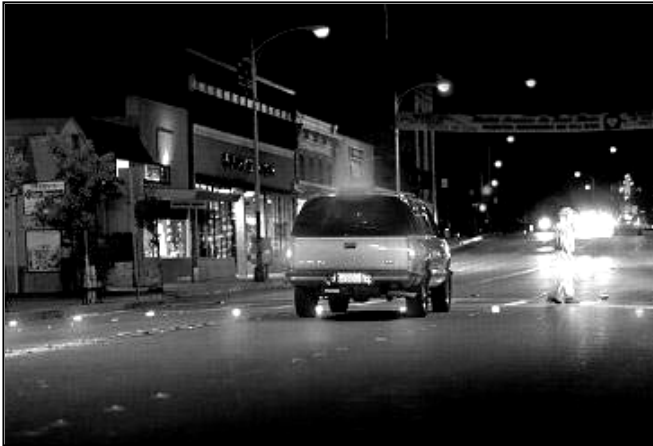
Figure 4.8 Overhead yellow flashing lights used at a zebra crossing in the US (Malek 2001)
