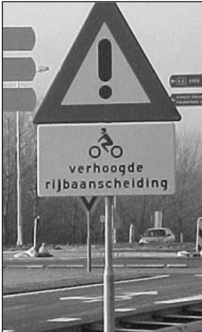
Figure 8.33 Advance warning sign for motorcyclists that reads 'Raised lane dividers' (Royal Haskoning 2009)
