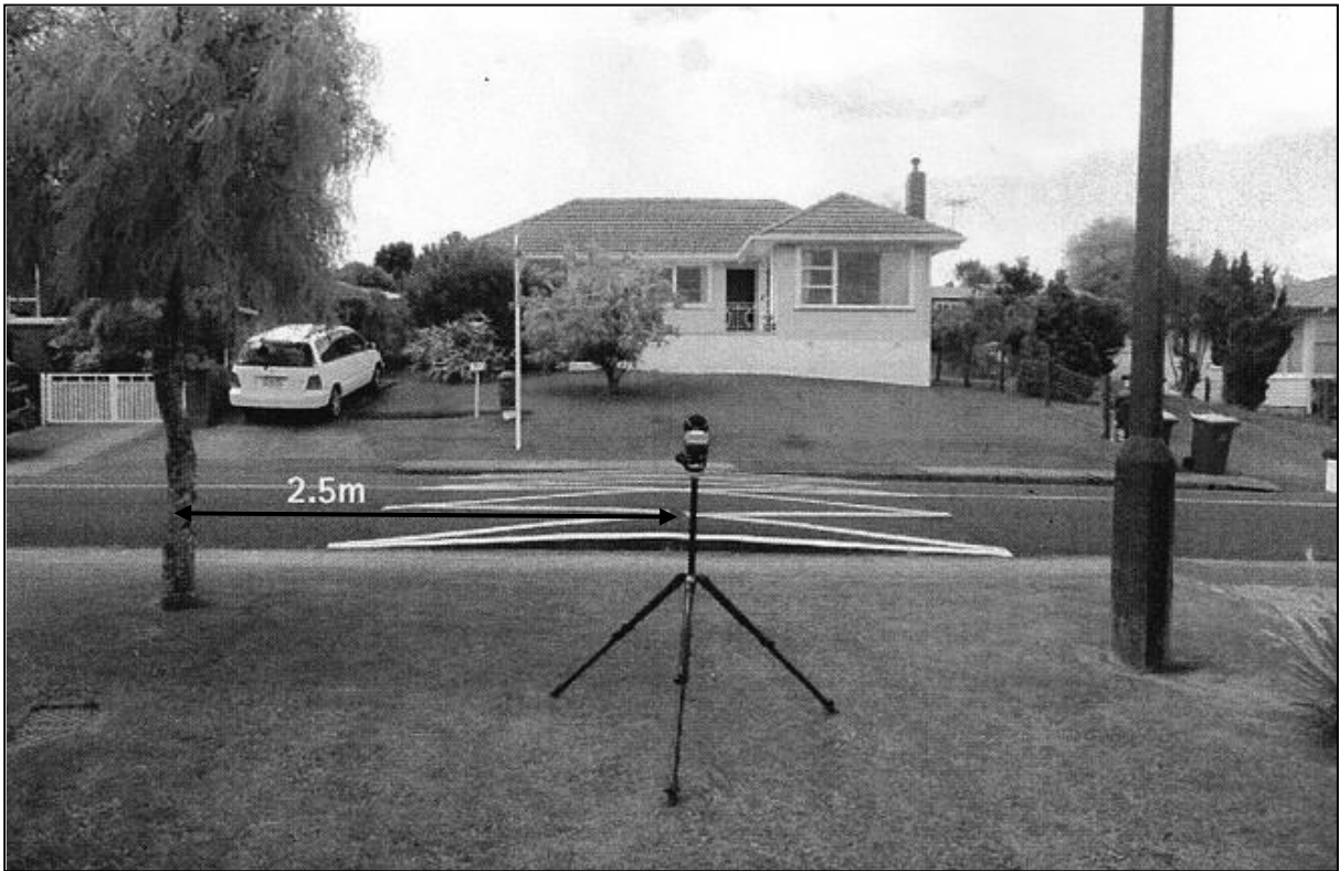
Figure 7.18 Photo showing the assessment site at Waitaki Street, Waitakere. The MWP speed hump is 5m long by 100mm high, and spacing was approximately 100m between each device
