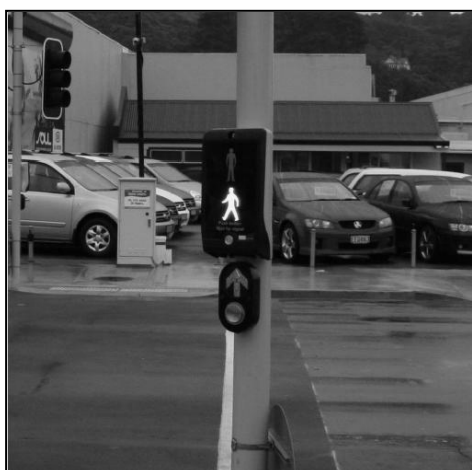
Figure 5.16 The nearside pedestrian displays that are a feature of the Puffin crossing recently trialled in Lower Hutt (King 2010)
