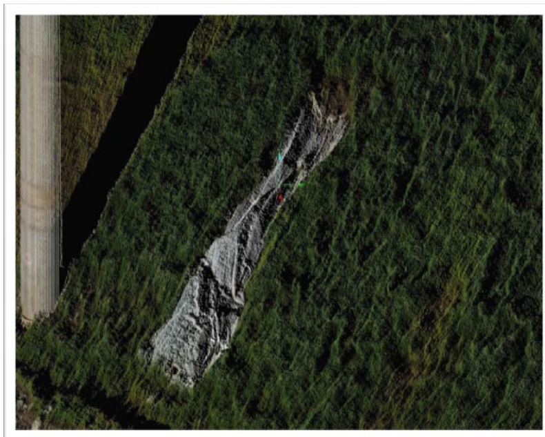
Figure 3.10: 3D laser scan point cloud of a shallow slope failure.
