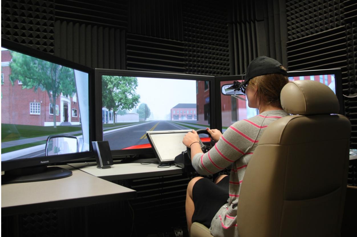
Figure 16. Participant in the driving simulator and wearing the eye tracker used in reported studies.
