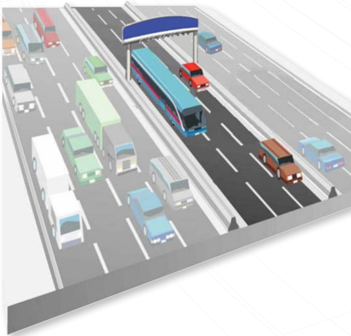
Figure 1: Example of BTL Adding New Capacity in the Median of a Limited-Access Highway with All-Electronic Tolls
