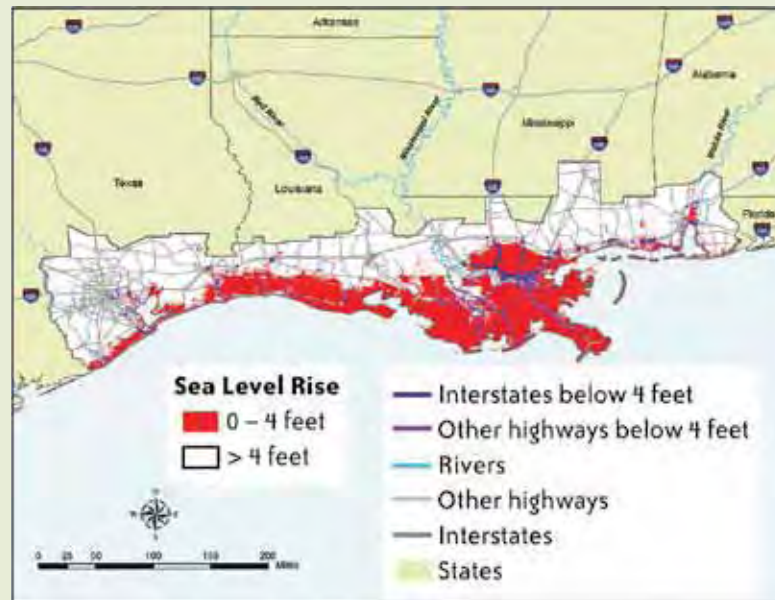
Figure 2.2 Gulf Coast Study: Highways Vulnerable to Relative Sea-Level Rise (RSLR) of Four Feet
