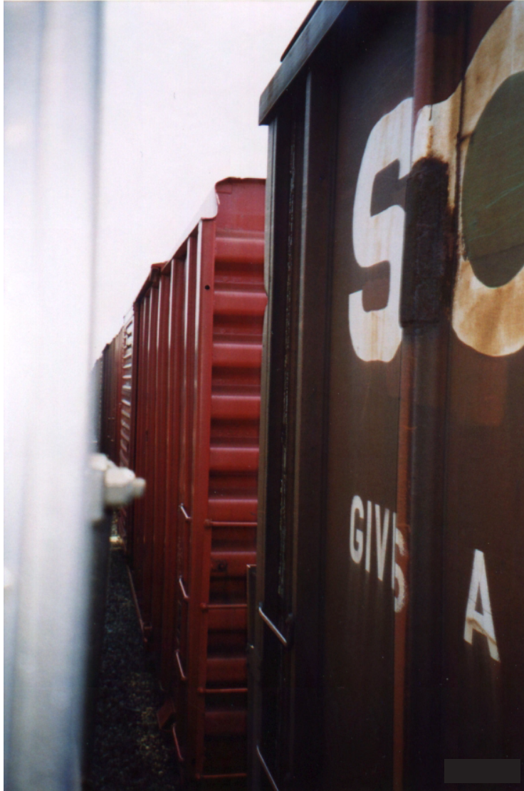
Figure 37. Example of close clearance between railroad tracks in a railroad yard
