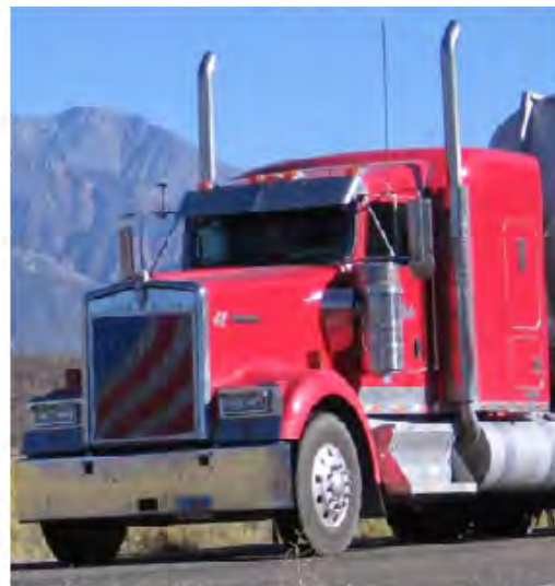
Typical classic styled truck with long nose, flat bumper, low-roof, and exposed air cleaners, exhaust stacks, and fuel tanks.
