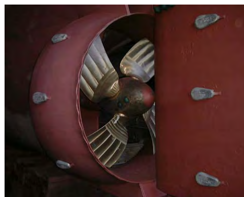
Figure 3.11 Nozzles Enclosing Propeller to Reduce Friction Losses
