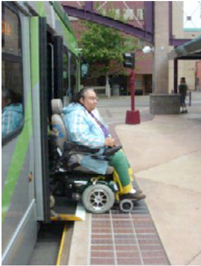
Figure 15 Wheelchair Customer Using Ramp to Board EmX
