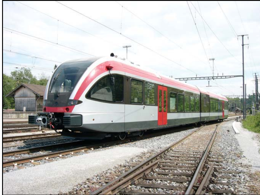
FIGURE 2 The Interurban car designated for use on Capital Metro–Austin. At 130 ft in length, and with operator crash protection, it is completely different in concept from the Media–Sharon Hill Line LRVs.
