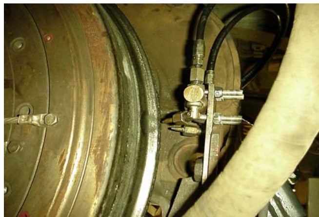
FIGURE 13 Onboard lubricator: flange lubricator on LRV117.
