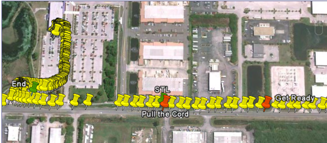
Figure 30 - TAD Prompts in Relation to the Second to Last (STL) and Ending (End) Bus Stops
