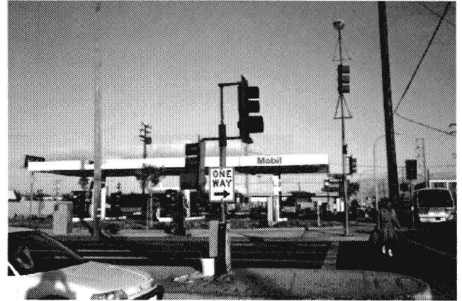
Median-mounted left turn signals before long mastarms became available Graphic - 3112
