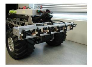
Figure 3: SHARP GP2D12 Infrared sensors for range detection.
