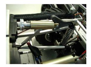
Figure 2: Cantilever suspension activated by a high torque servo rotating the piston screw.
