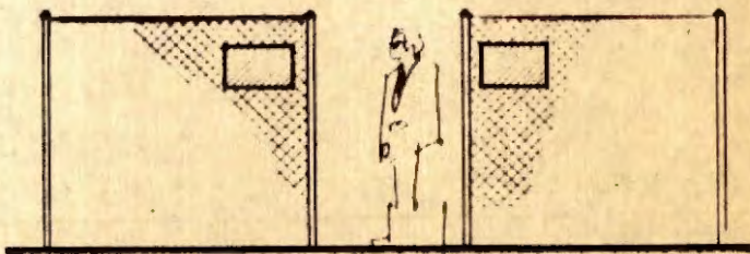
14 Information Plaque Mounted to Fence 15 Restrictive Plaque Mounted to Fence
