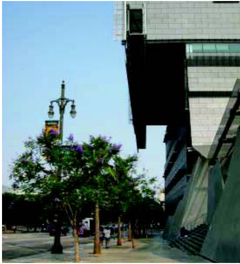
Examples of building overhang that does not interfere with street tree growth.
