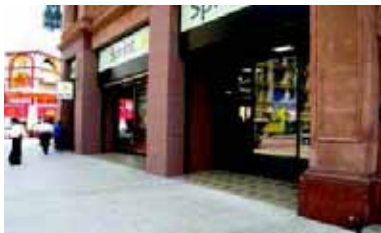
The Bradbury Building's columns and upper story walls are within a foot of the back of the required sidewalk, while entrances and display windows are setback a few feet.
