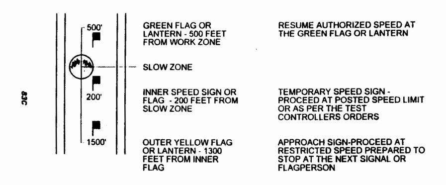
NOTE: SHOULD A PASSENGER STATION BE LOCATED WITHIN THE LIMITS OF THE PROTECTED (FLAGGED) ZONE, AN ADDITIONAL YELLOW FLAG SHALL BE PLACED AT THE DEPARTING END OF THE STATION PLATFORM.
