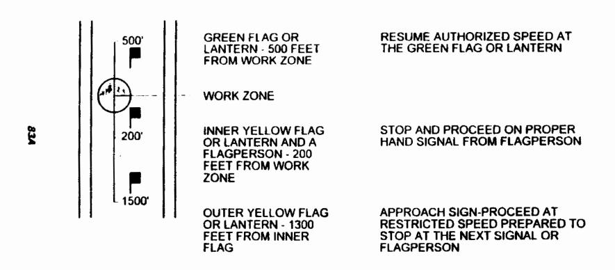
NOTE: SHOULD A PASSENGER STATION BE LOCATED WITHIN THE LIMITS OF THE PROTECTED (FLAGGED) ZONE, AN ADDITIONAL YELLOW FLAG SHALL BE PLACED AT THE DEPARTING END OF THE STATION PLATFORM.
