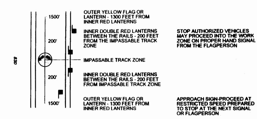
NOTE: SHOULD A PASSENGER STATION BE LOCATED WITHIN THE LIMITS OF THE PROTECTED (FLAGGED) ZONE, AN ADDITIONAL YELLOW FLAG SHALL BE PLACED AT THE DEPARTING END OF THE STATION PLATFORM
