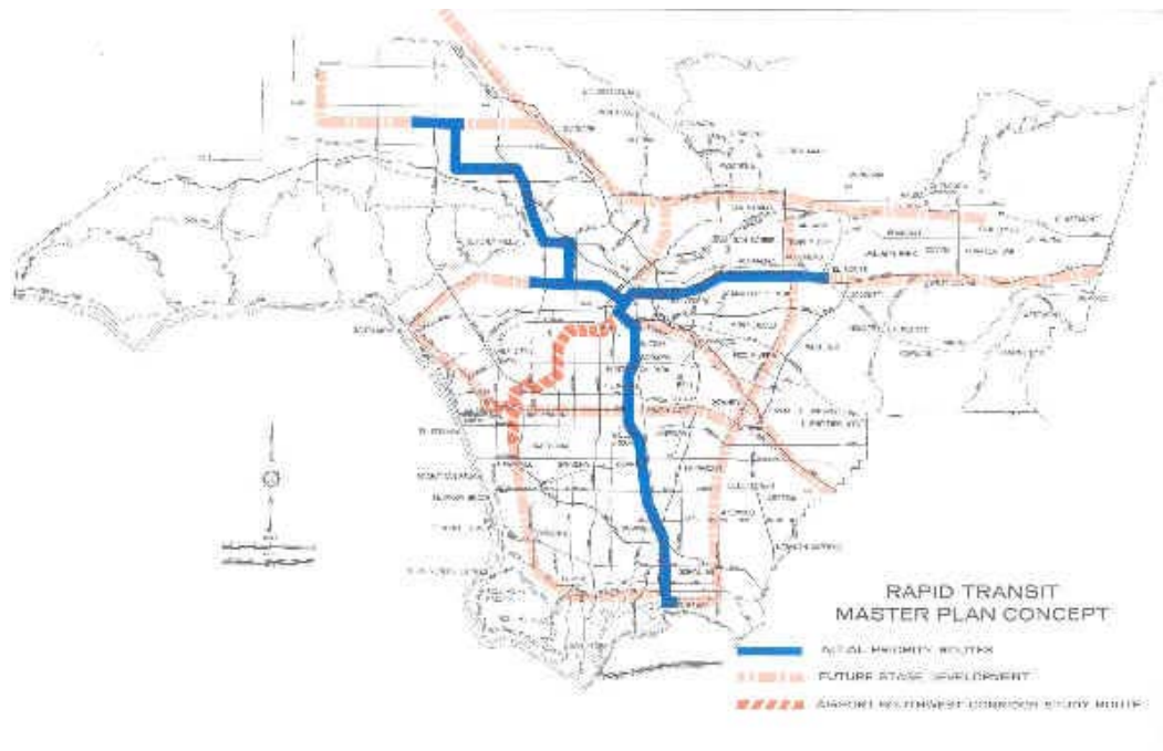
1968 Final Proposed Transit Master Plan Concept for a ballot initiative: Initial 62 mile four corridor system that could expand to 300 miles, projected cost of $2.5 billion, 8.5 year construction period:
