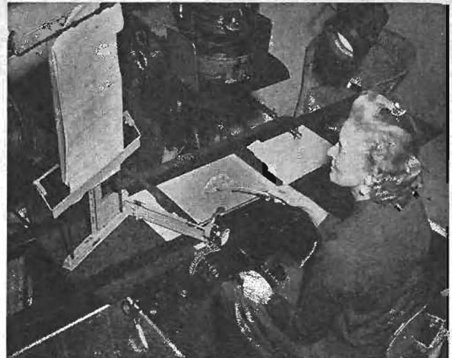
SHEET OF PAPER at upper left shows exact sequence of cells and frames. Laura holds air nozzle which blows dust from cells.
