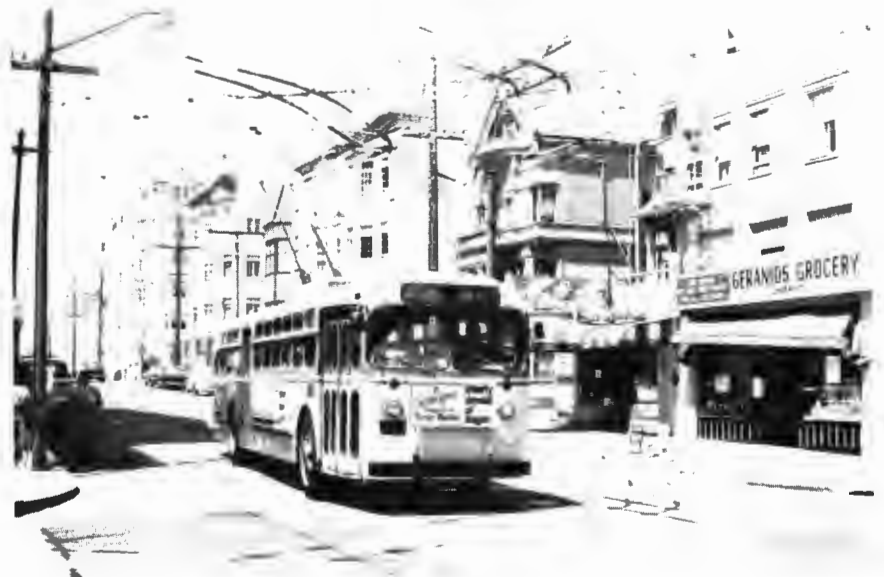
550-569, 660-739 : 44 pas- senger Marmon-Herrington trolley coach 728 at Cal- ifornia and Jackson on Line 22--FILLMORE.
