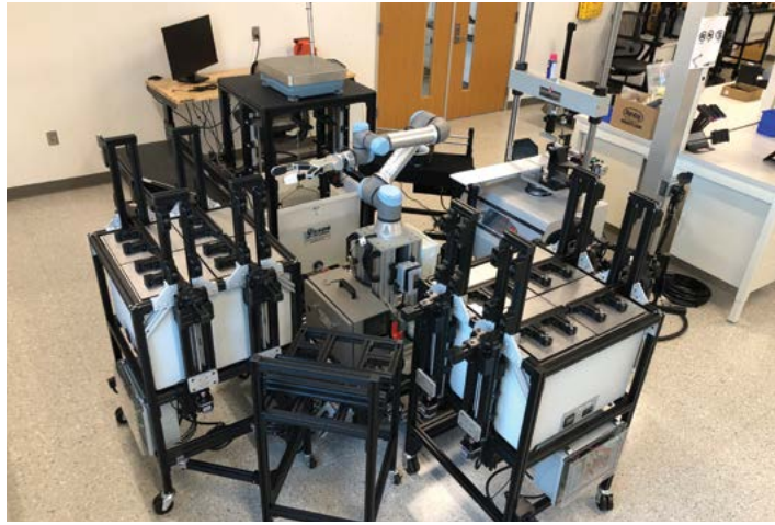
Asphalt mixture automated testing system with zero intervention (AMAZE). Photograph by Fujie Zhou, Texas Transportation Institute.
