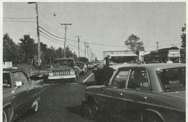
Figure J-9. Turn bays and shorter cycles can sometimes avoid multiple phases.
