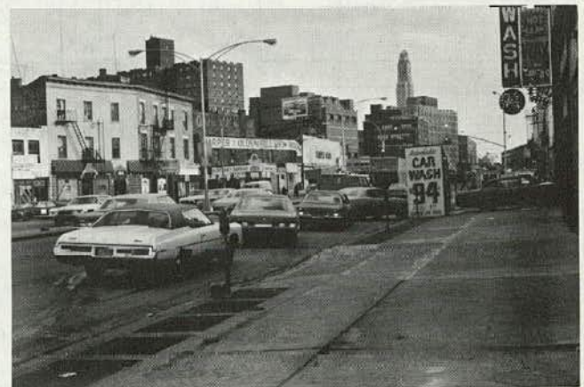
Figure J-32. Lane lost by standing queues on right-of-way.
