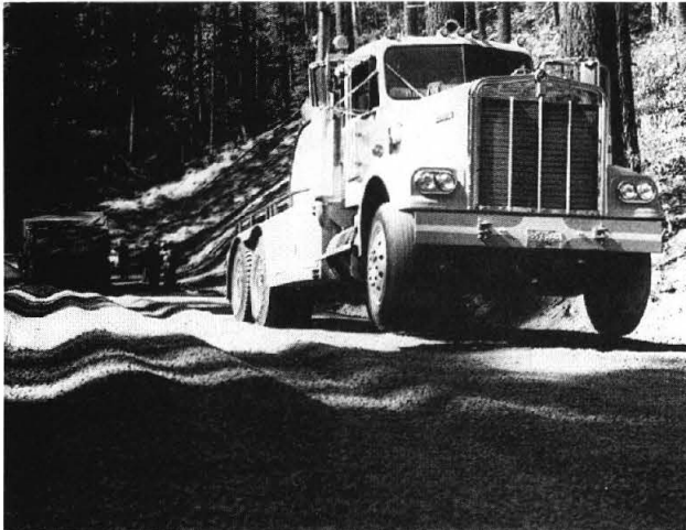
Figure 25 Tow truck front wheels lifted off the ground during removal of embedded truck.
