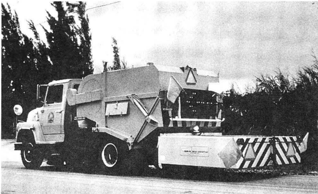
FIGURE 10 TMA Application with sweeper. (Courtesy EASI)
