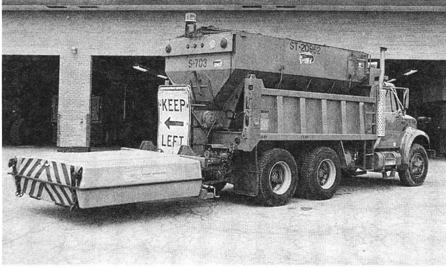
FIGURE 9 TMA Application with salt-spreader vehicle. (Courtesy SHRP)
