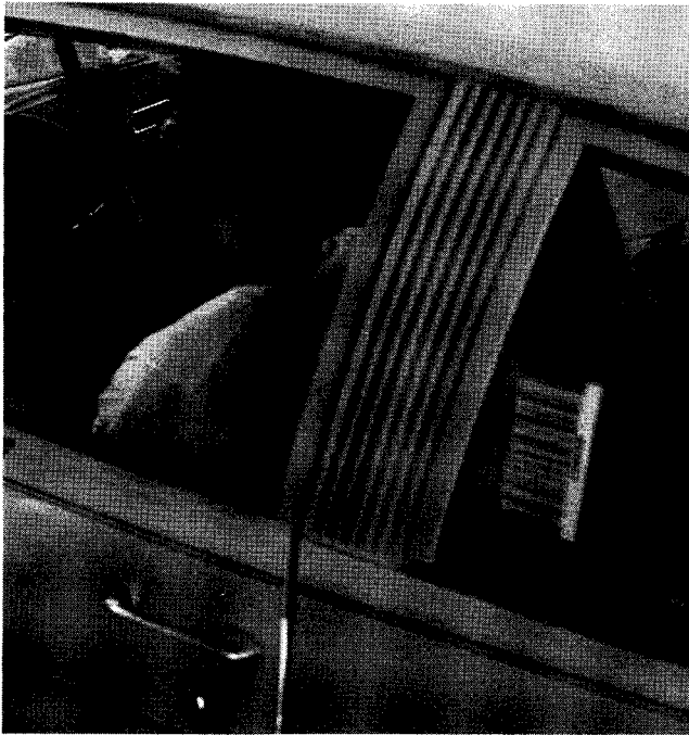
FIGURE 2 A bar code sticker affixed to the left rear window is read by a laser scanner as the vehicle approaches Bay Harbour Island just north of Miami.
