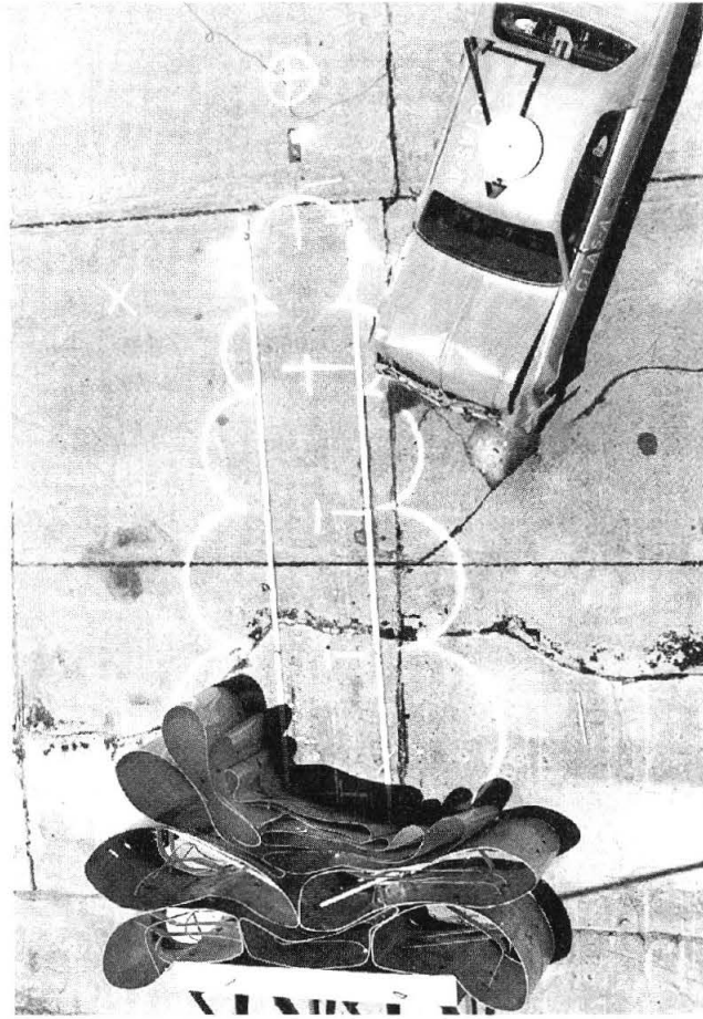
Figure 26 The GCIAS after impact.
