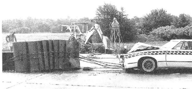
Figure 6b Impact result of a 100 km/h head-on collision by 2,041 kg automobile.
