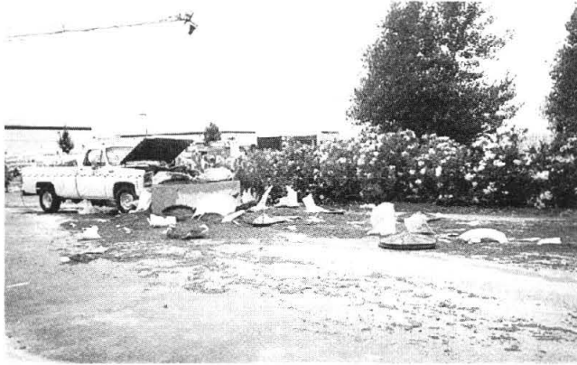
Figure 15 Sand-filled plastic barrel crash cushion after impact. (Courtesy of Energy Absorption Systems, Inc.)
