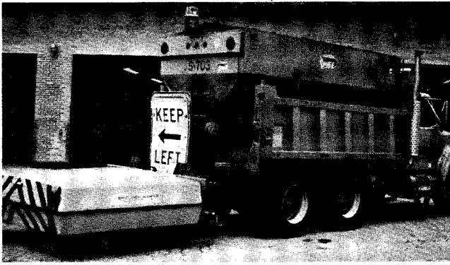
FIGURE 17 Truck-mounted impact attenuator for spreaders, developed by SHRP.
