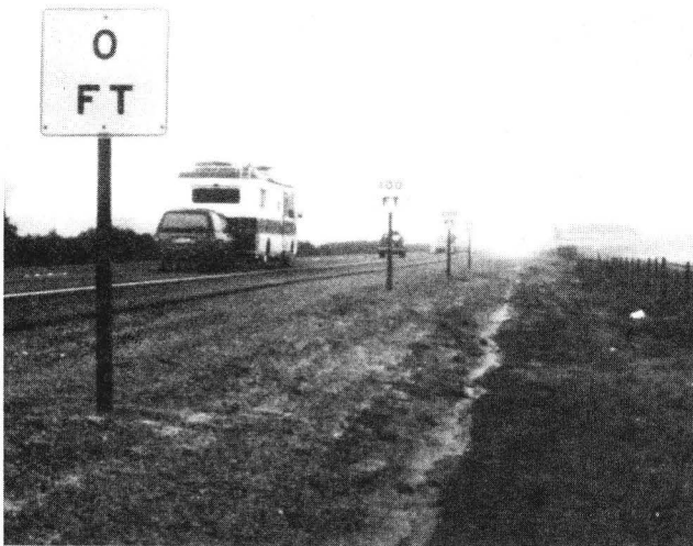
FIGURE 5 Fog visibility test sign.
