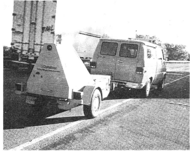
FIGURE 1 Dynatest 8000 falling weight deflectometer owned by Oklahoma DOT.
