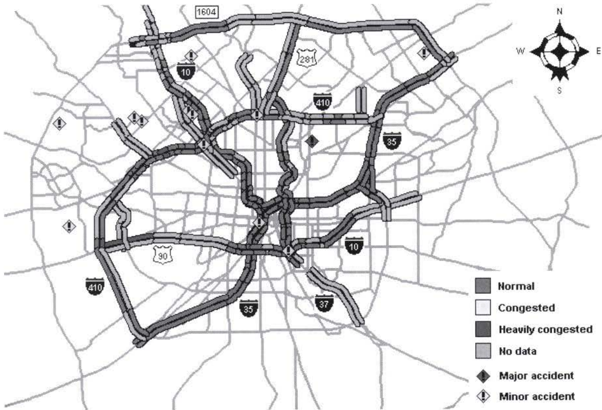
FIGURE 6 The Texas DOT-San Antonio District TransGuide web site provides information of current incidents and alternate routing on San Antonio freeways in real time. (Graphic courtesy of the Texas DOT.)
