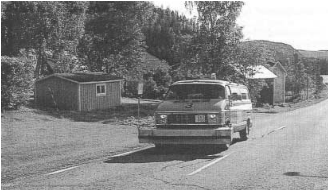
Figure 13. Infrastructure Management Services Laser RST profiler.
