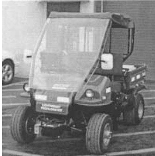
Figure 25. K.J. Law T6450 lightweight profiler.
