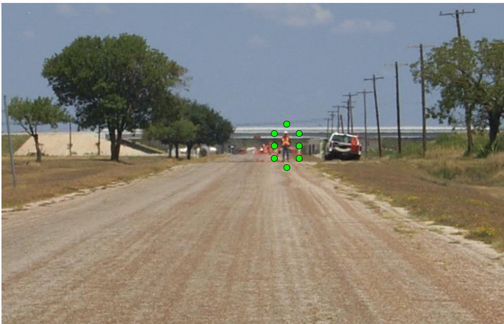
Figure 30. Background Luminance Measurement Locations.
