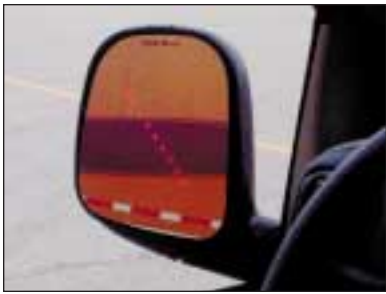
A collision warning sensor with a lighted graphic link to the rear view mirror detects obstacles in the adjacent lane.
