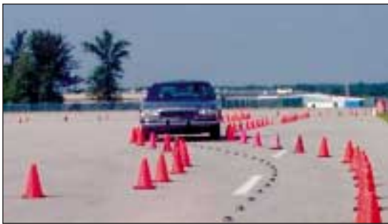
Lane tracking devices with magnets along a test route.
