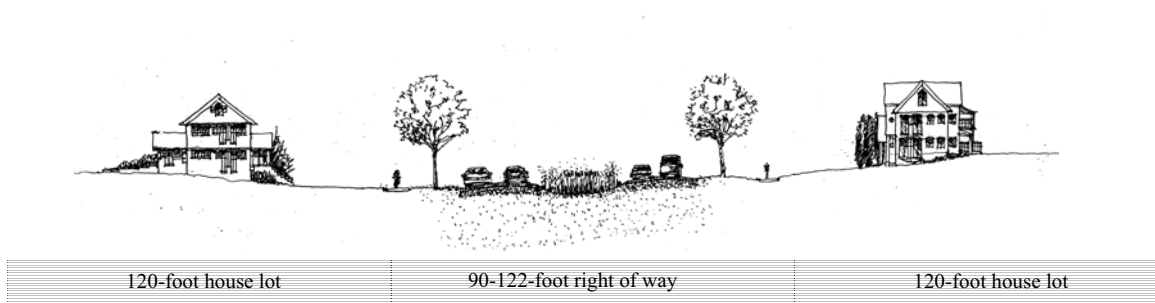
Figure 10.12 Intermediate Street: Four-lane Divided CROD-Lo/CROD Med/Hi Parkway
