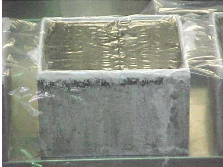
Figure 2.2: Concrete slab undergoing ponding
