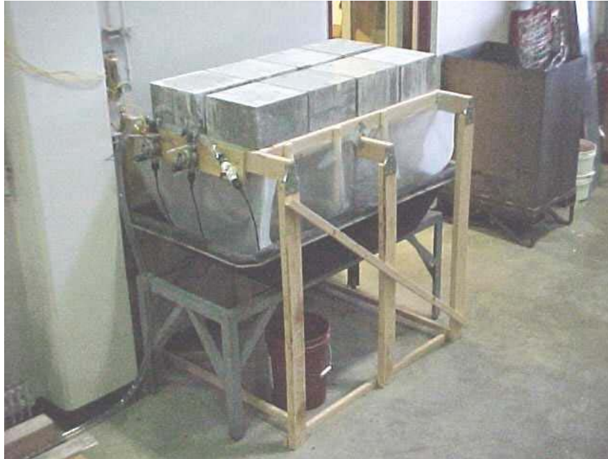
Figure 2.3: Rack for washing slabs
