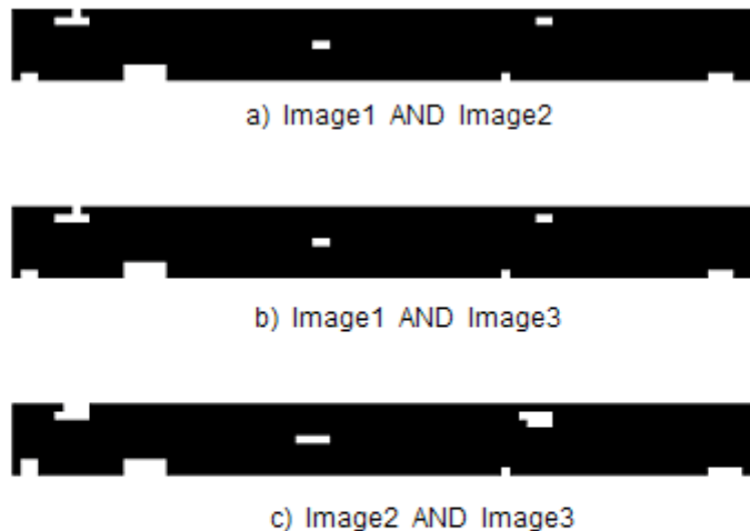
Figure 4.13 Common Objects taken from Pair of Binary Images (from fig. 4.12) a) New_Image1 = Image1 AND Image2 b) New_Image2 = Image1 AND Image3 c) New_Image3 = Image2 AND Image3
