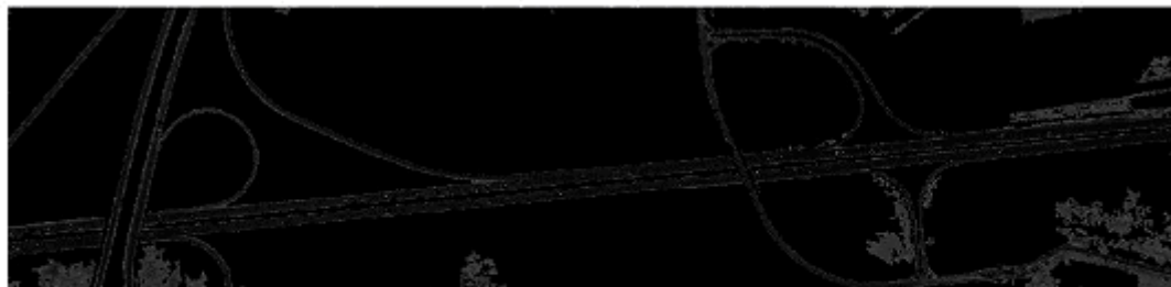
Figure 3.4 Intensity Image obtained after applying the algorithm to detect highways to the image in figure 3.1a)
