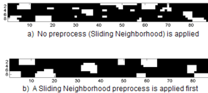
Figure 4.15 Binary Images obtained by applying the Otsu Threshold a) No preprocess step is applied b) A preprocess step is applied first
