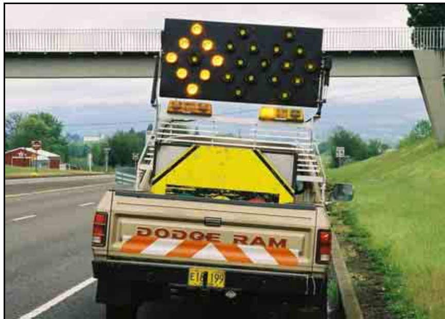
Figure 4.1: Type B Arrow Panel Display Mounted on ¾-ton Truck
