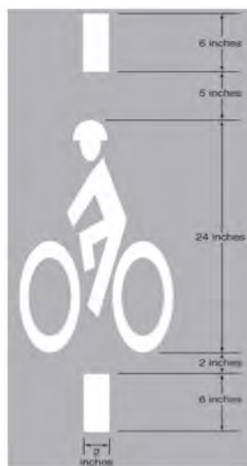
Figure A0-2 Bicycle Detector Pavement Marking
