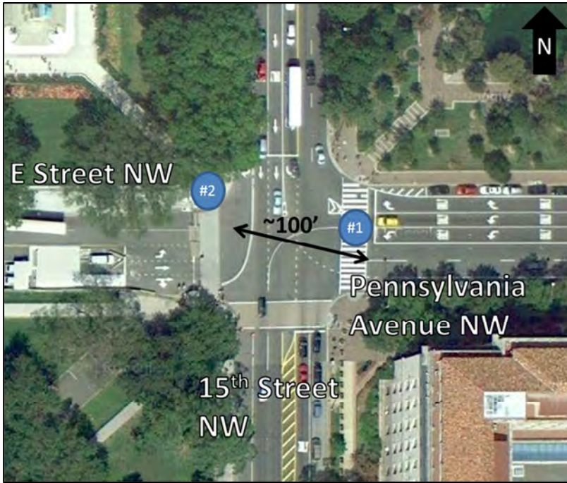
Figure 1. Approximate Crossing Distances and Bike Signal Locations (does not show bike infrastructure)
