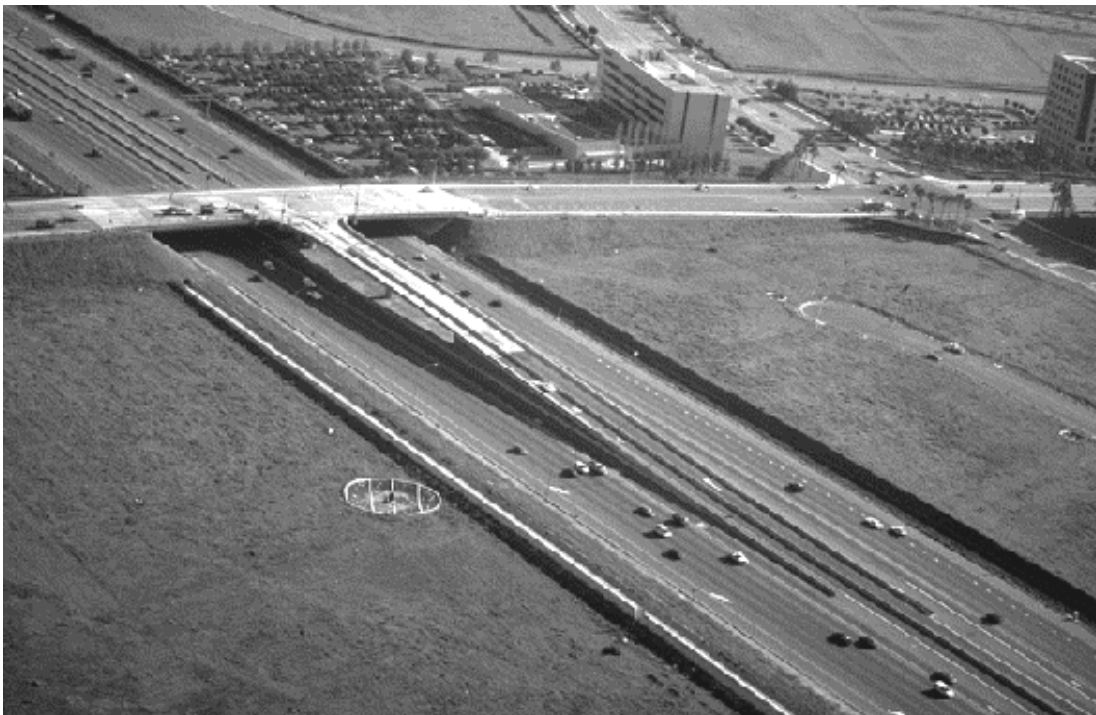
Figure 11. Drop Ramp in Orange County, California (2).
