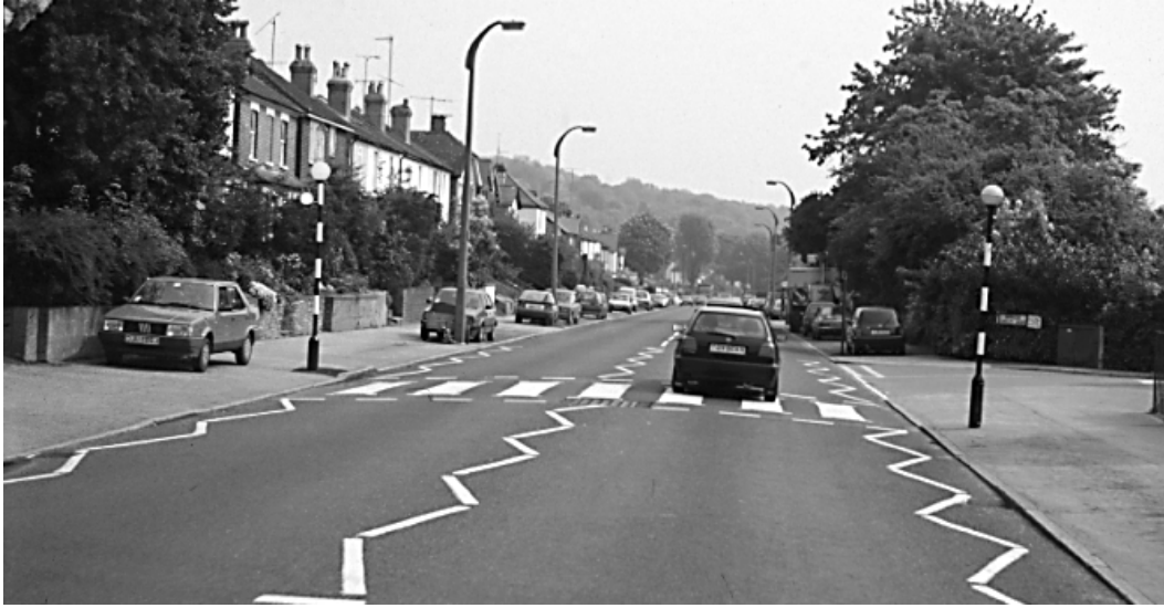
Figure 29. Use of Zig-Zag Lines and Belisha Beacons to Warn of Upcoming Pedestrian Crossing – United Kingdom (19).
