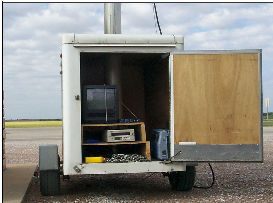
Figure 4. Internal View of Video System Trailer.
