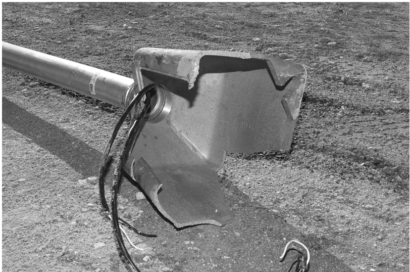
Figure 15. Installation after Test 417920-2.
