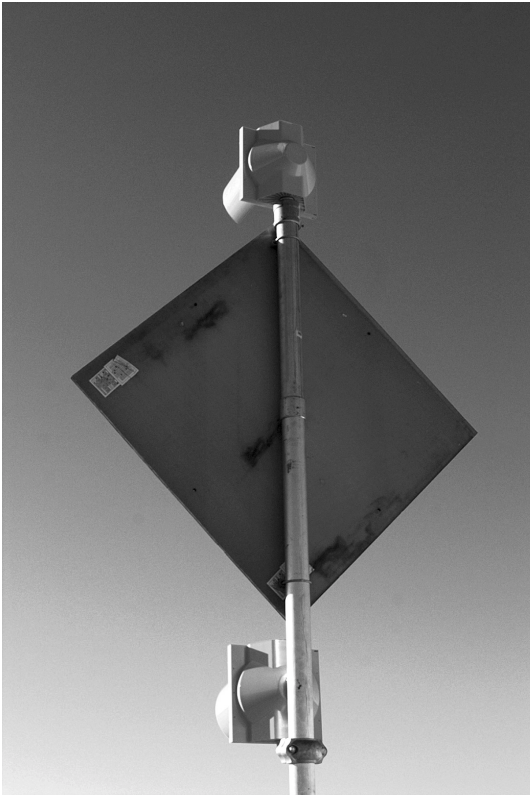
Figure 3. Pedestal Base Sign Support before Test 417920-1.
