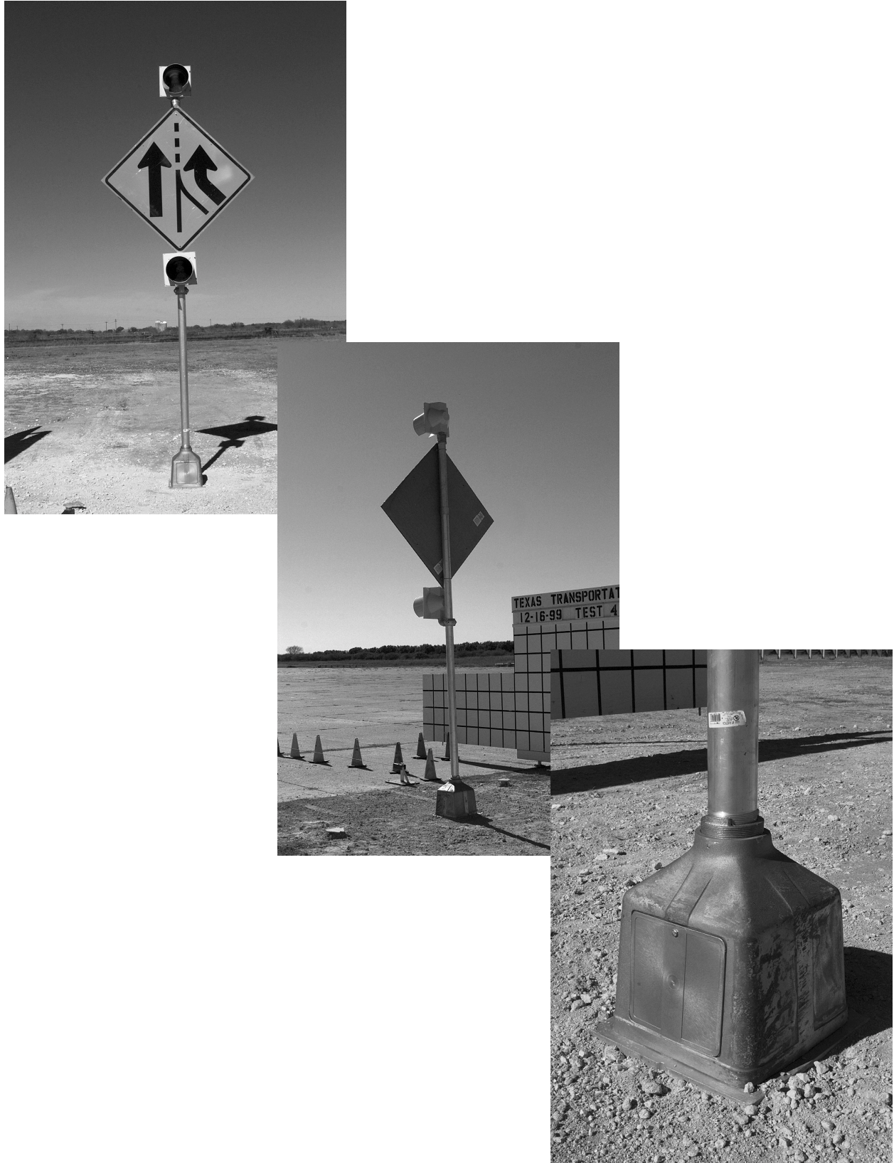
Figure 4. Pedestal Base Sign Support before Test 417920-2.
