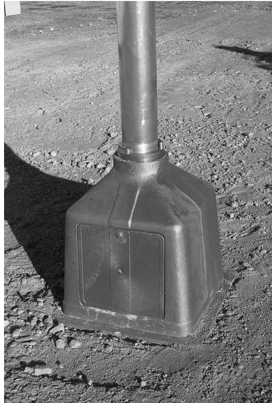
Figure 3. Pedestal Base Sign Support before Test 417920-1.
