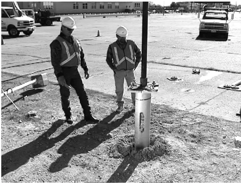
Figure 2. Installation of Anchor Used in Tests 417920-1 and 417920-2.
